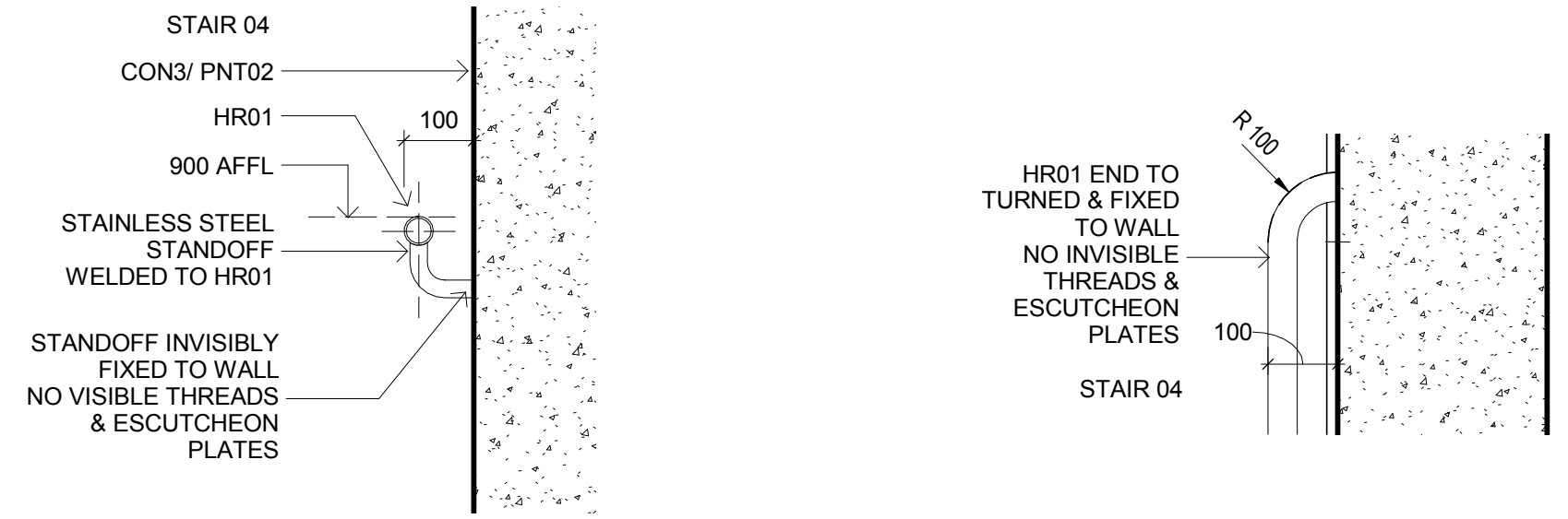
3 HR01 WALL FIXED - SECTION DETAIL 1:10
