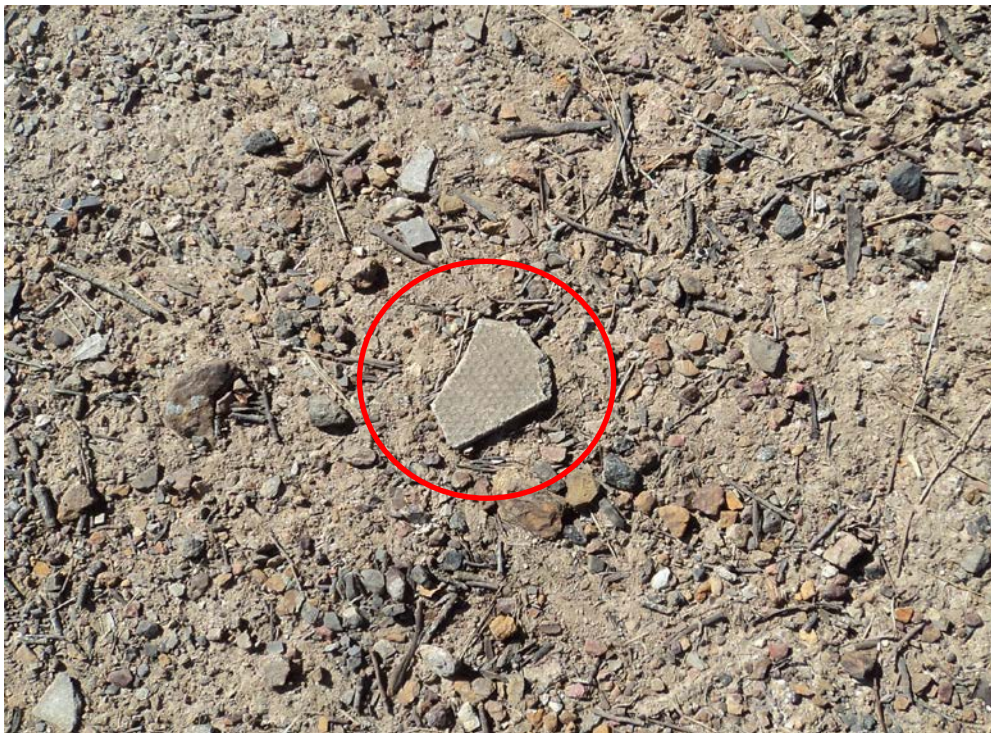
Photo 6 - Fibre-cement fragment observed on ground surface
