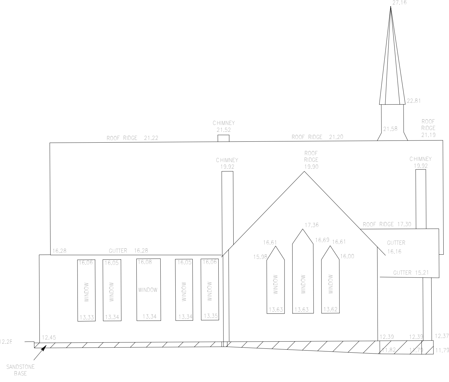
2 HERITAGE B - EXISTING - EAST ELEVATION 1:100
