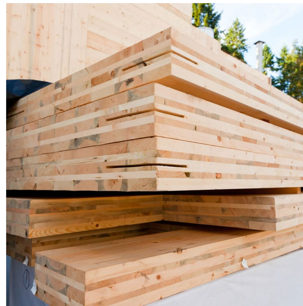
Cross Laminated Timber Panels
