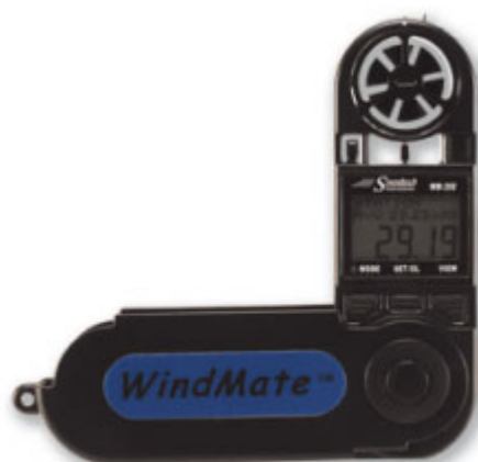
Figure B-1 Typical hand-held wind meter
