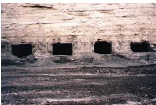
Figure 3: An example of a highwall mining operation (Galvin, 2016).
