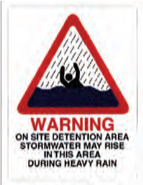
OSD WARNING SIGN N.T.S SUGGESTED SIZE 600mm x 450mm TO BE PROVIDED ADJACENT TO OSD TANKS IN SUITABLE AREA T.B.C ON SITE
