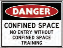
CONFINED SPACE SIGN N.T.S SUGGESTED SIZE 300mm x 450mm TO BE PROVIDED ADJACENT TO OSD TANKS IN SUITABLE AREA T.B.C ON SITE
