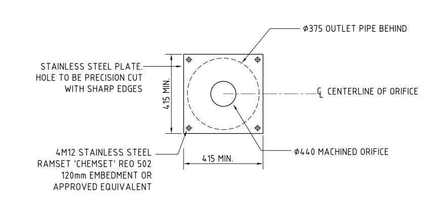
OUTLET- ORIFICE PLATE DETAIL SCALE 1:10
