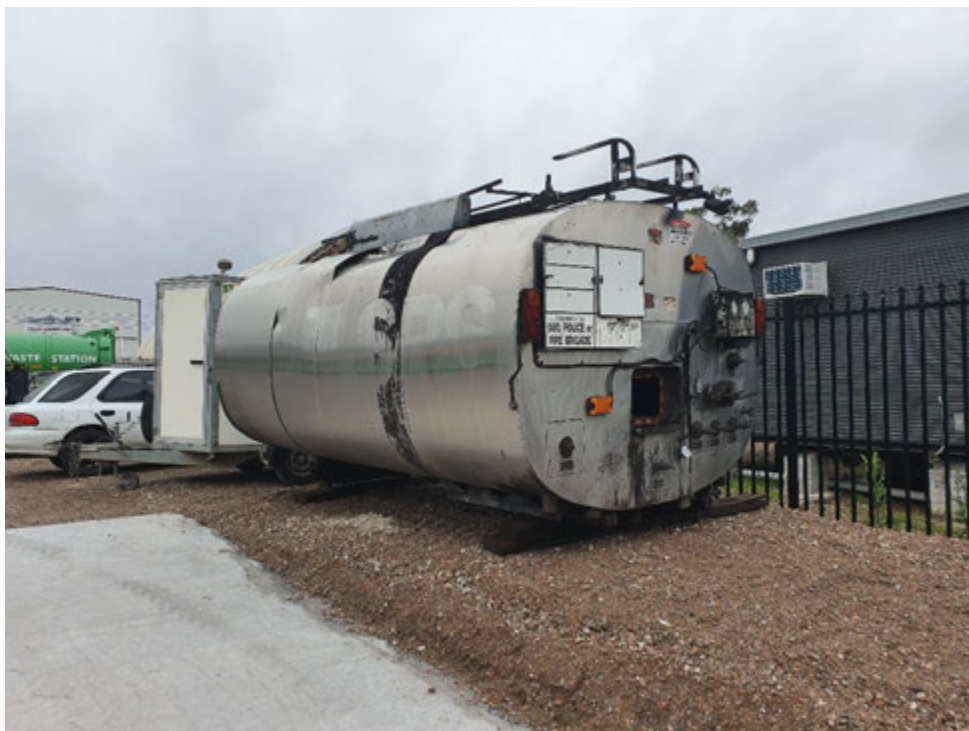
Photograph 2 – Stored vehicle storage tank which appears to have bitumen store within previously. No staining was evident on the ground surrounding or beneath the tank.
