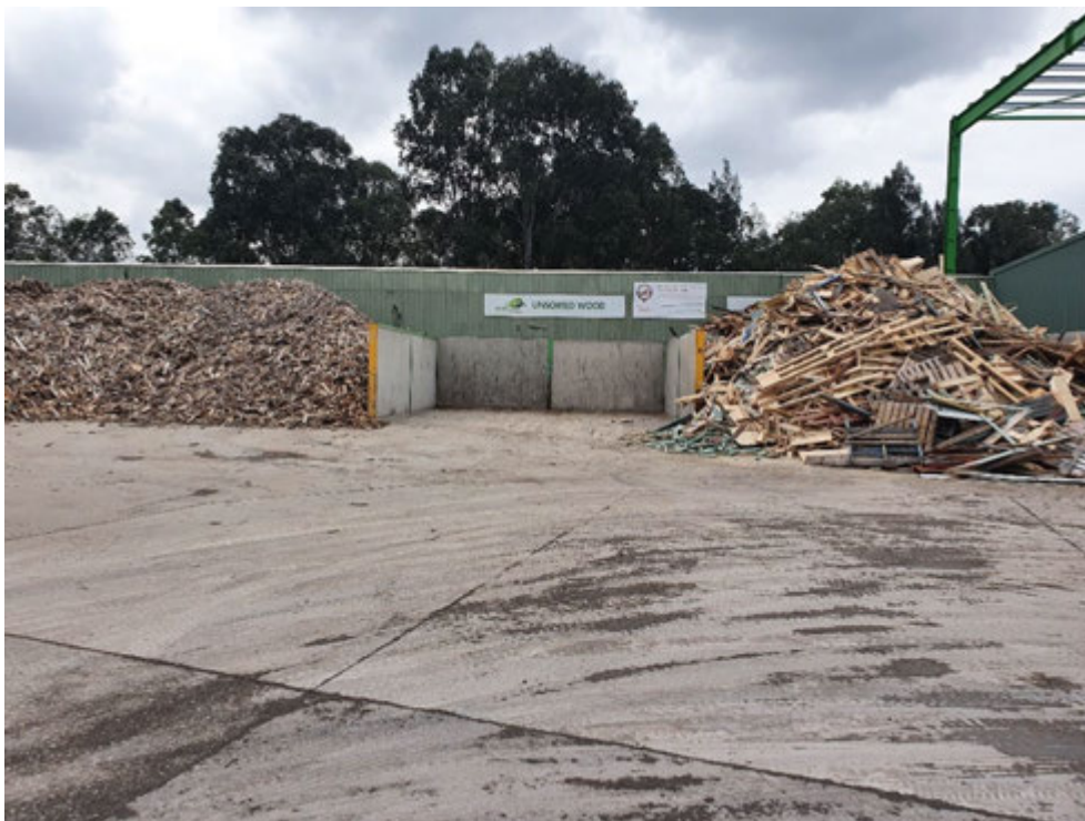
Photograph 4 – (8 Styles St) Timber storage bays where various timber types are segregated prior to processing.
