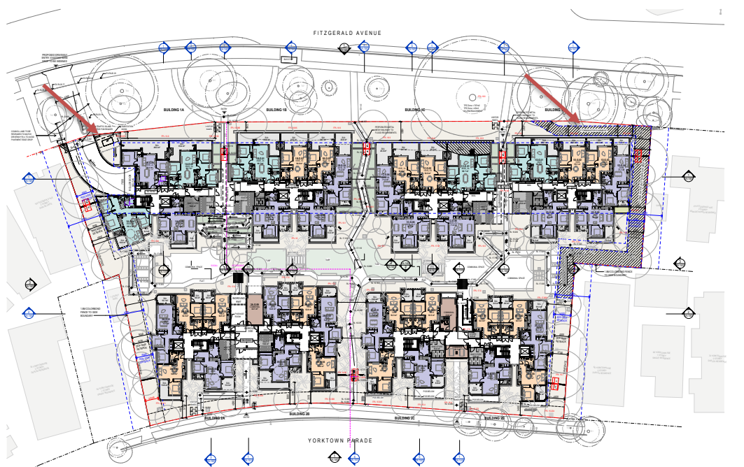
Figure 1 –The Ground Floor plan showing Ausgrid electrical kiosk now within site boundary (arrowed top left) and the building relocated south of the original position in the north eastern corner (arrowed top right). (Source: Hayball November 2025)
