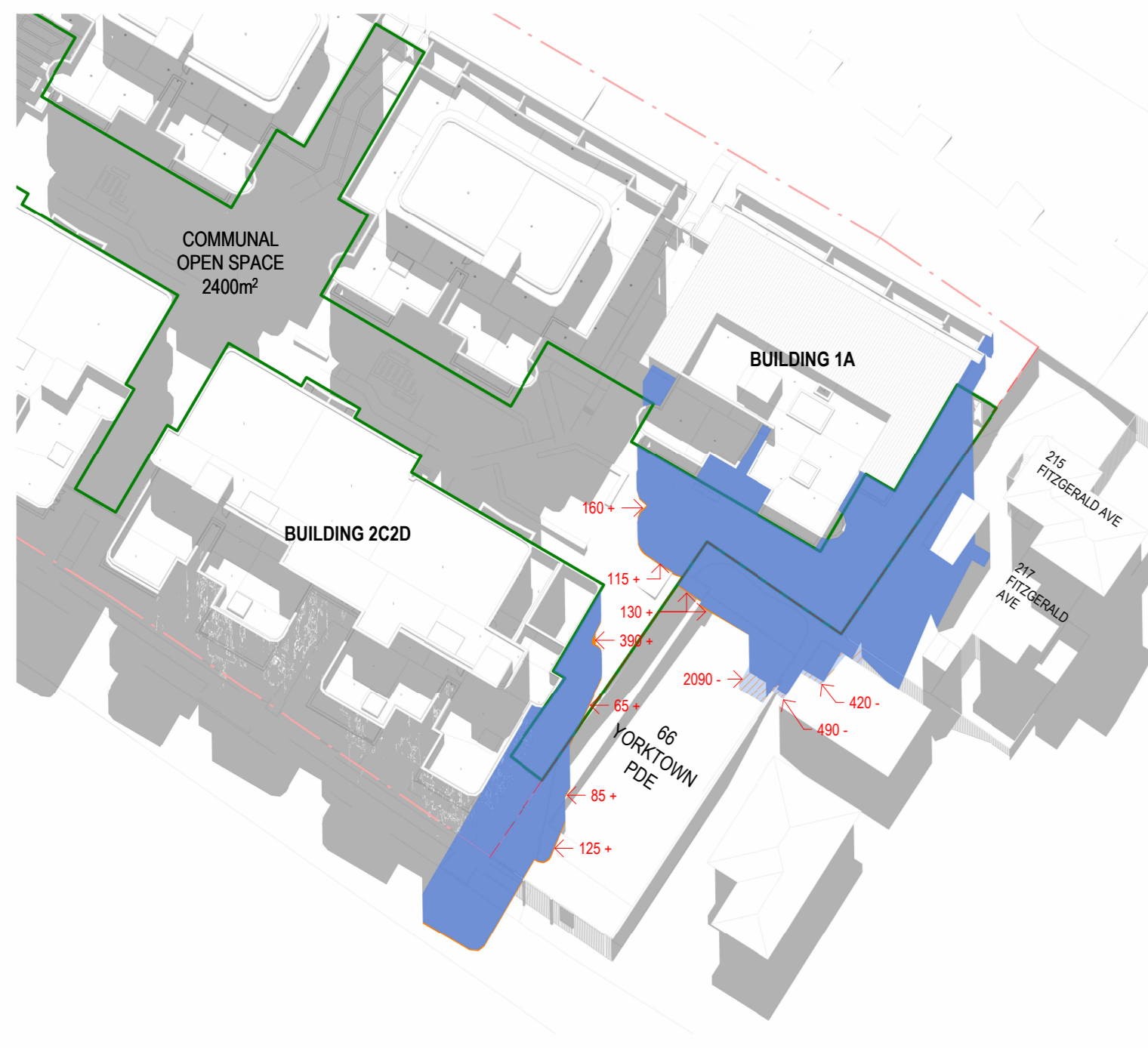
4 PLAN WINTER SHADOW DIAGRAM - 21 JUNE 12PM SCALE 1 : 600
