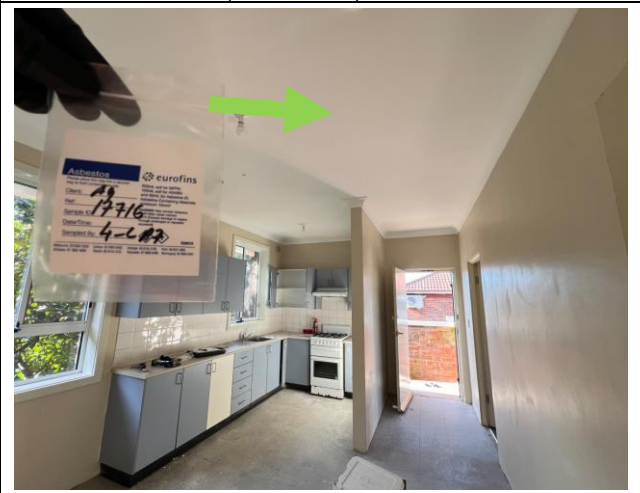
Photograph 10 (20.06.24): Representative photo of white paint system, internal kitchen and hallway ceiling, Sample ID: 4-LP7 (< 0.01 % w/w)
