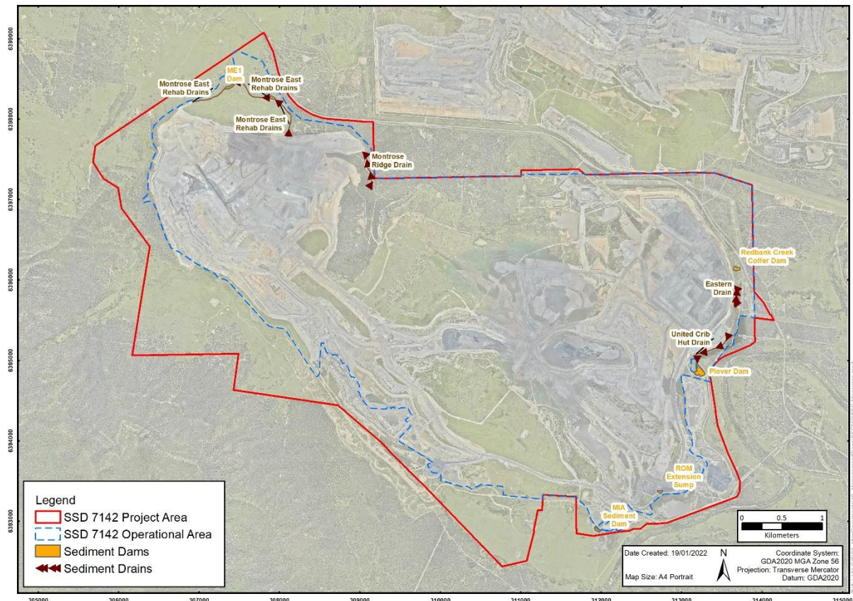
Figure 9-2: Key Erosion and Sediment Control Measures
