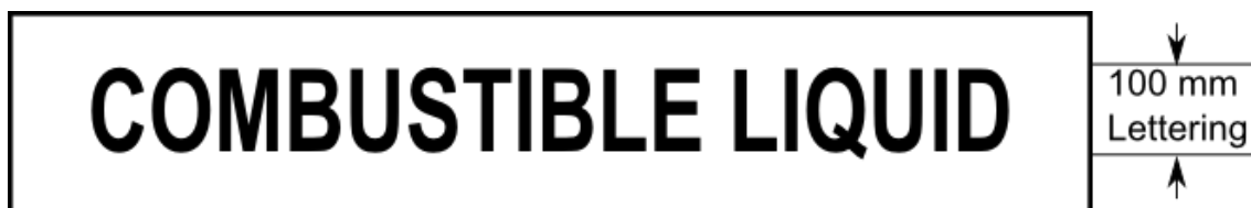
Figure 5-2: Combustible Liquid Placard
