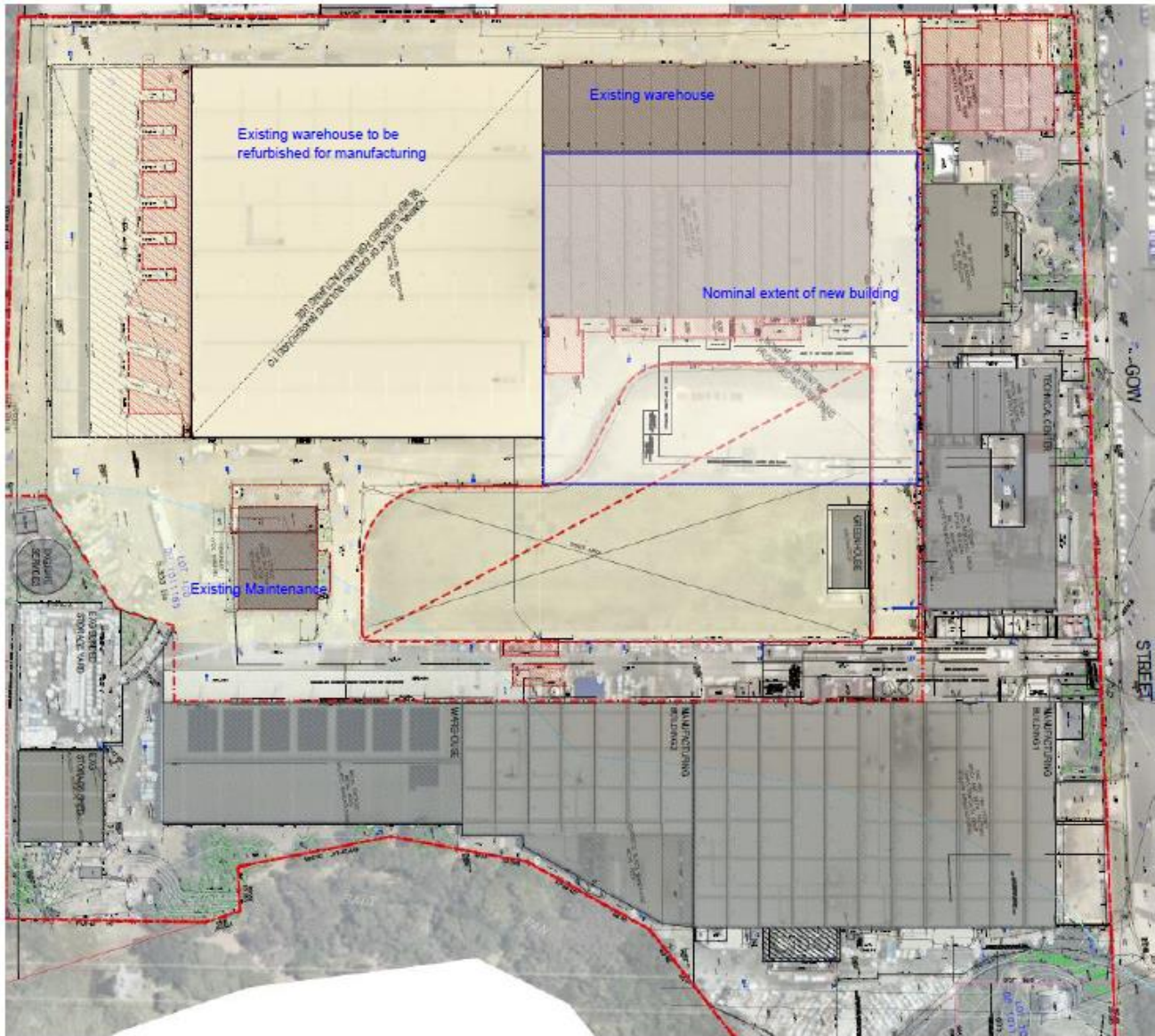
Figure 5. Existing site layout showing demolition works in red hatched areas and the nominal extent of the new building. (North is on right hand side of drawing)
