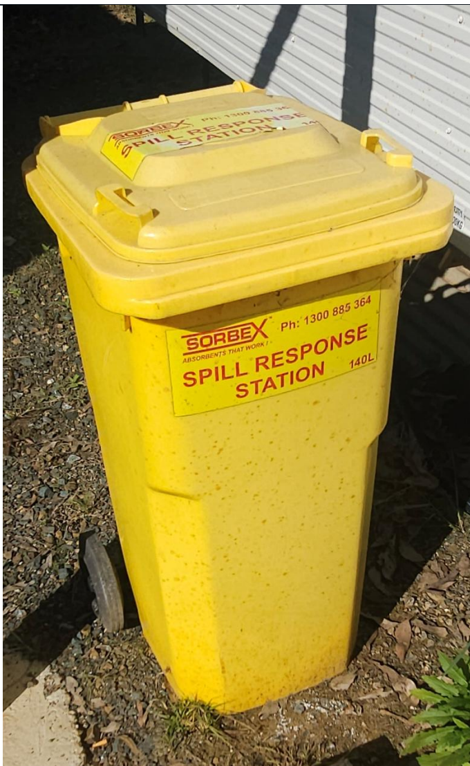
Plate 2 Spill response kit at site compound
