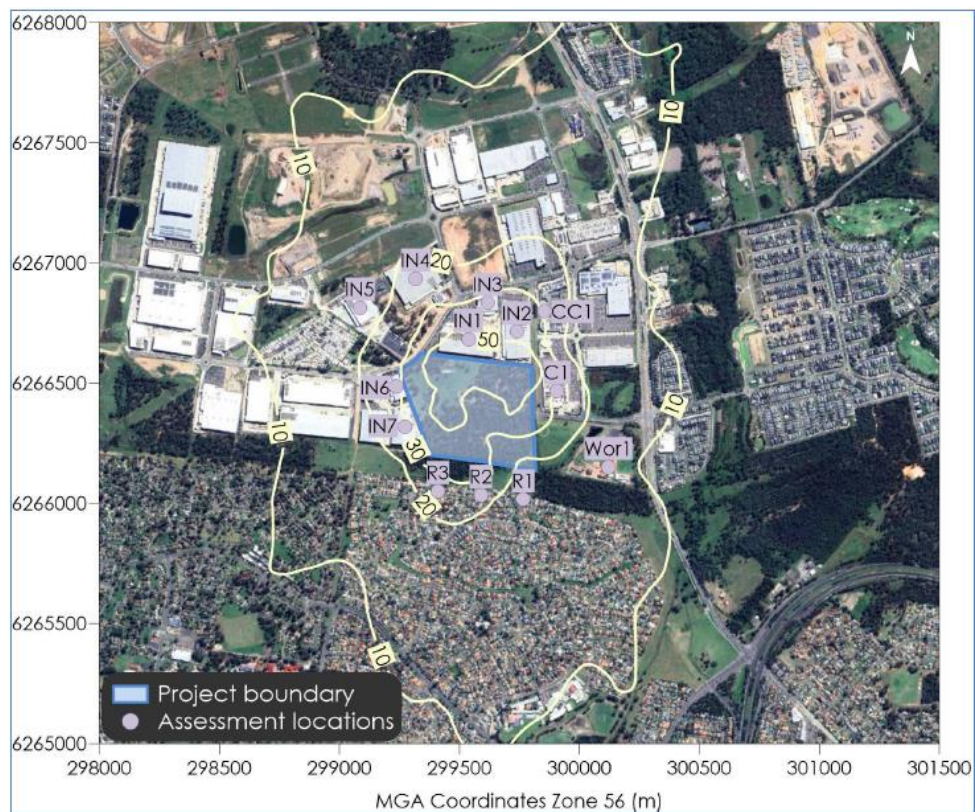
Figure 52: Scenario 1 Predicted incremental 24hr average PM 2.5 concentrations (µg/m 3 ) Source: Air Quality Impact Assessment – Todoroski
