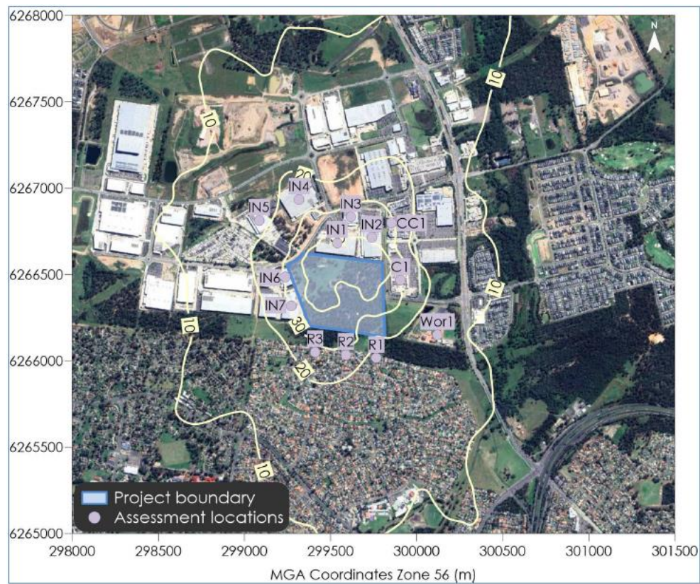
Figure 53: Scenario 1 Predicted incremental 24hr average PM 10 concentrations (µg/m 3 ) Source: Air Quality Impact Assessment – Todoroski
