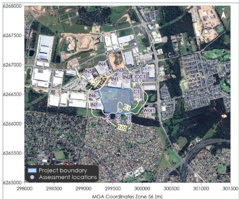
Figure 58: Scenario 2 Predicted incremental 24-hour average PM 10 concentrations due to emissions from annual testing (µg/m 3 )
