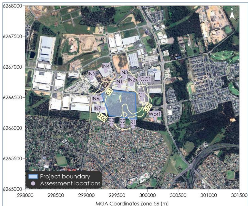
Figure 56: Scenario 2 Predicted incremental 24-hour average PM 2.5 concentrations due to emissions from annual testing (µg/m 3 )
