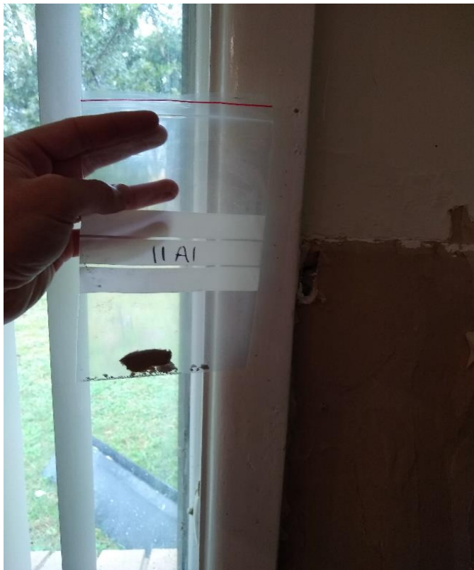
Photo 5: Building 11, interior, wall sheeting in eastern bedroom in house, plaster sheeting, sample 11A1, no asbestos detected by analysis.
