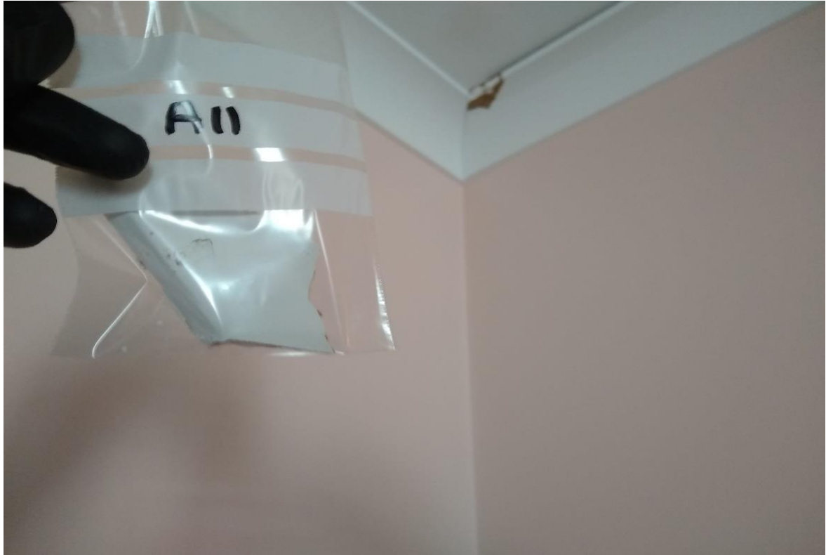
Photo 11: Building 24, interior, wall sheeting in bathroom in house, plaster sheeting, sample 24A1, no asbestos detected by analysis (SMF detected).
