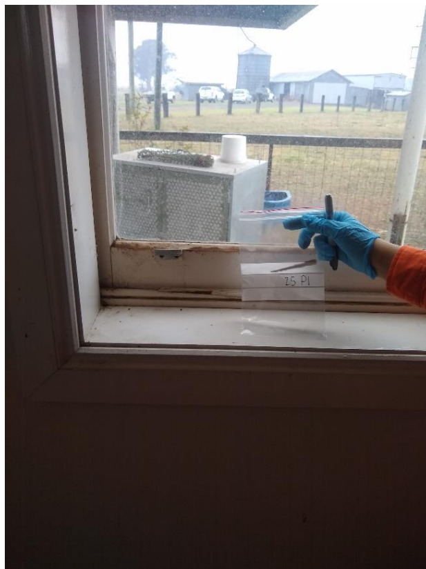
Photo 36: Building 25, interior, paint off timber window frame in northern bedroom in house, white paint, sample 25L1, no lead paint(s) identified
