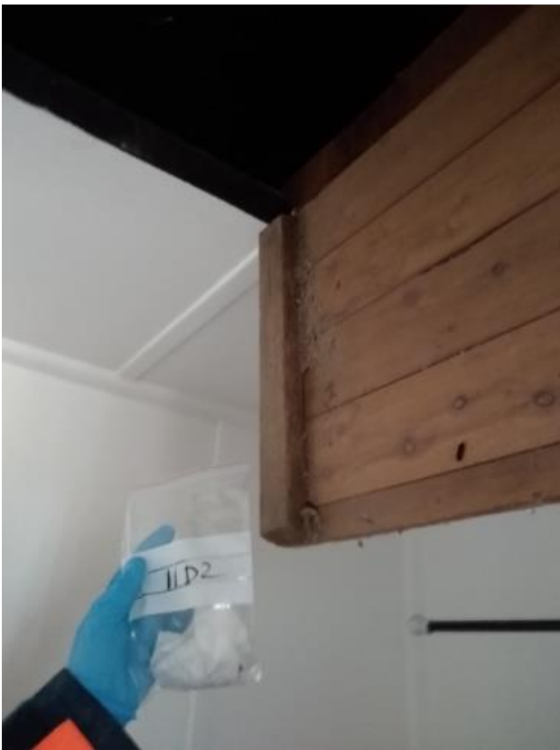
Photo 50: Building 11, manhole in western portion of house, throughout, settled dust, sample 11D2, lead concentration <0.5 mg/m2
