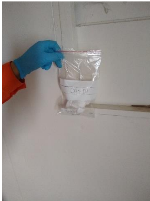
Photo 54: Building 34, timber window sill in central portion of structure, throughout, settled dust, sample 34D1, lead concentration <0.5 mg/m2
