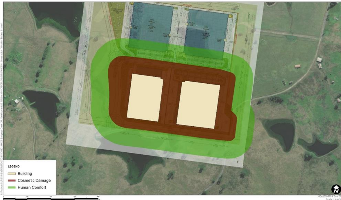
Figure 6 Construction Vibration – Large Vibratory Roller
