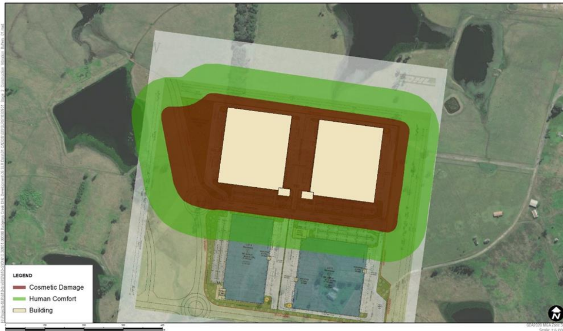
Figure 6 Construction Vibration – Large Vibratory Roller
