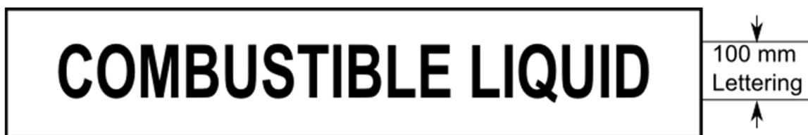
Figure 5-2: Combustible Liquid Placard
