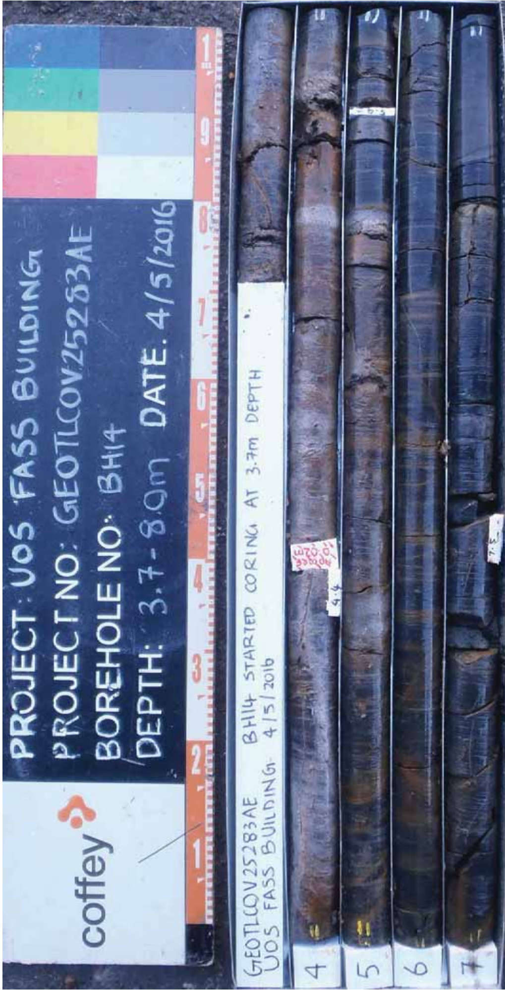
PointID : BH14 Depth Range: 3.70 - 8.00 m
