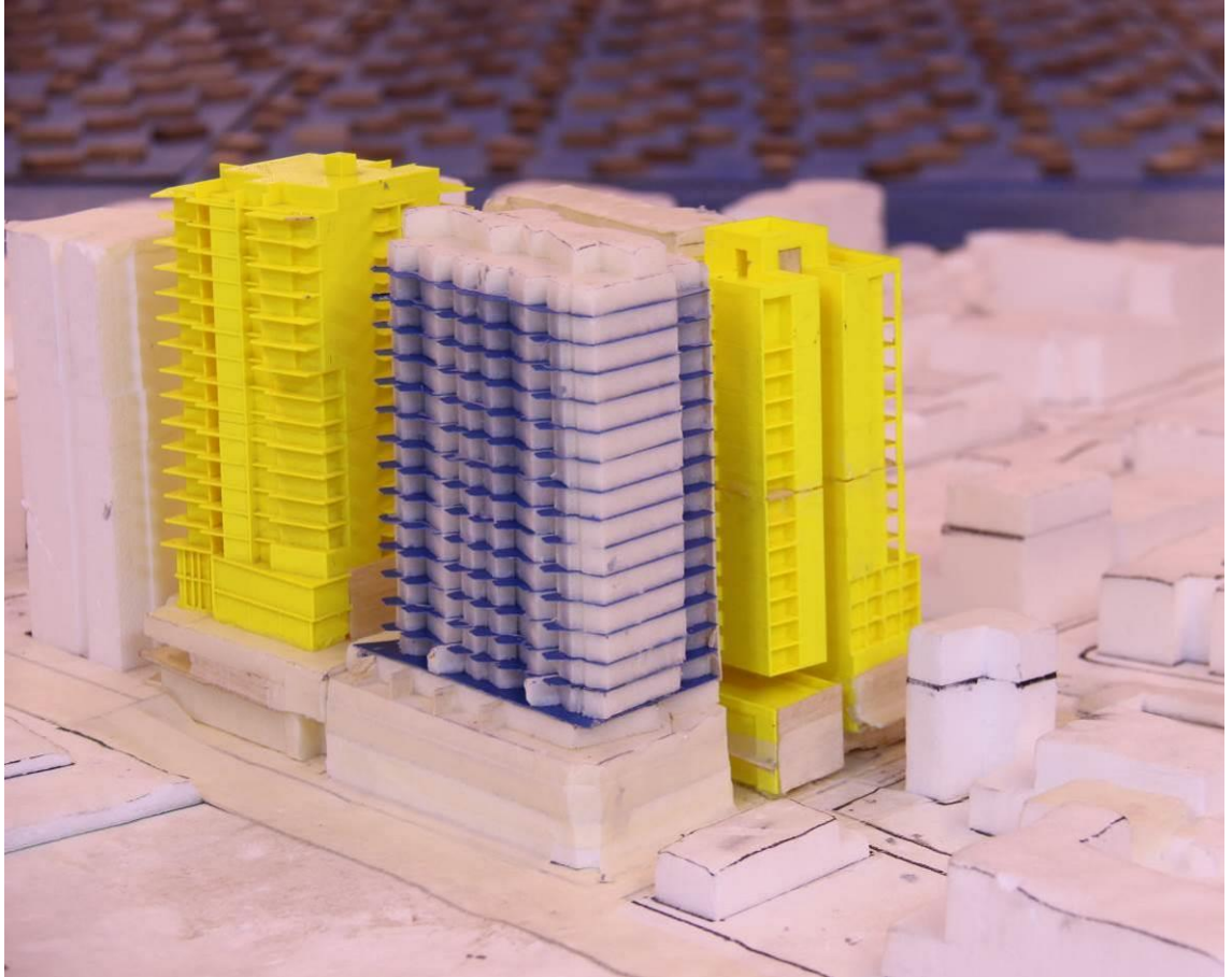
Figure 2h: Photograph of the Wind Tunnel Model (close up view from the south-west)
