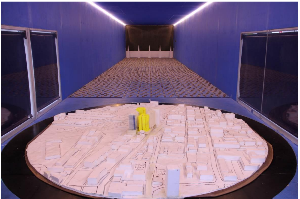
Figure 2a: Photograph of the Wind Tunnel Model (view from the south)
