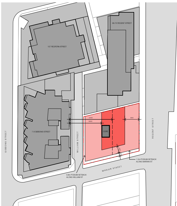
02. Existing podium and tower setbacks as per SEPP (Major Developments) and SEPP 65 results in non-developable floor plate
