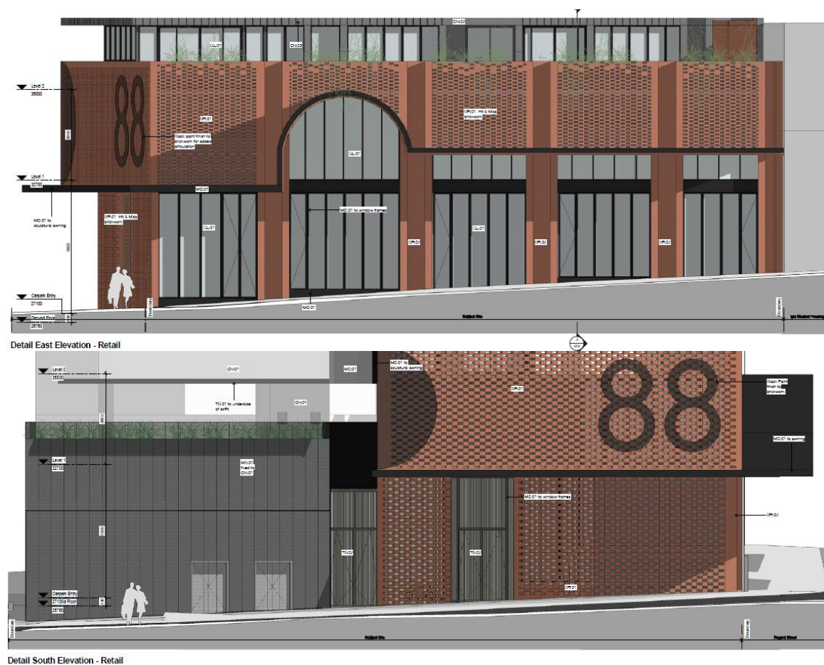
Figure 16: Expression and materiality of the ground level
