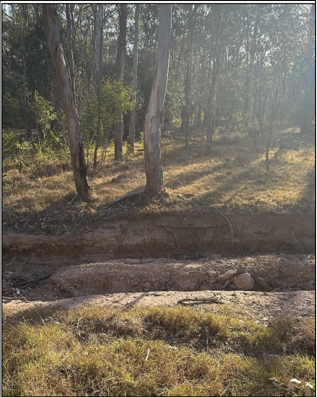
N33: NSA – exposed surficial soils and residual clays in area of rutting
