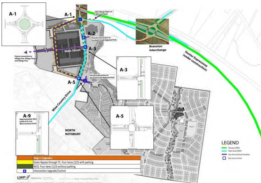
Figure 7a: Detail of road and intersection upgrades
