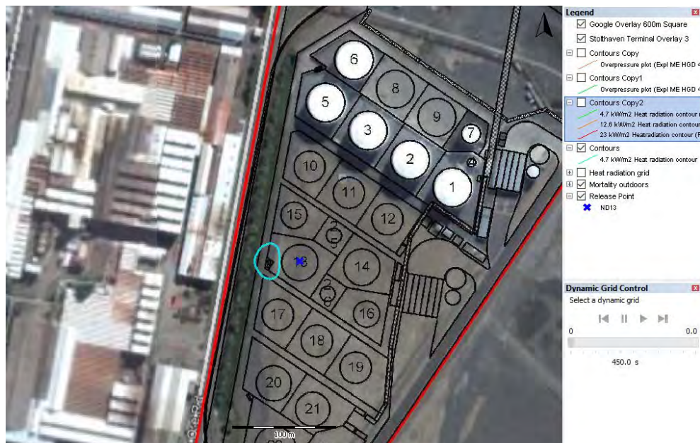
Figure 1 Single Tank-top fire, ND16 – heat radiation of 4.7 kW/m 2 at 1.5m height
