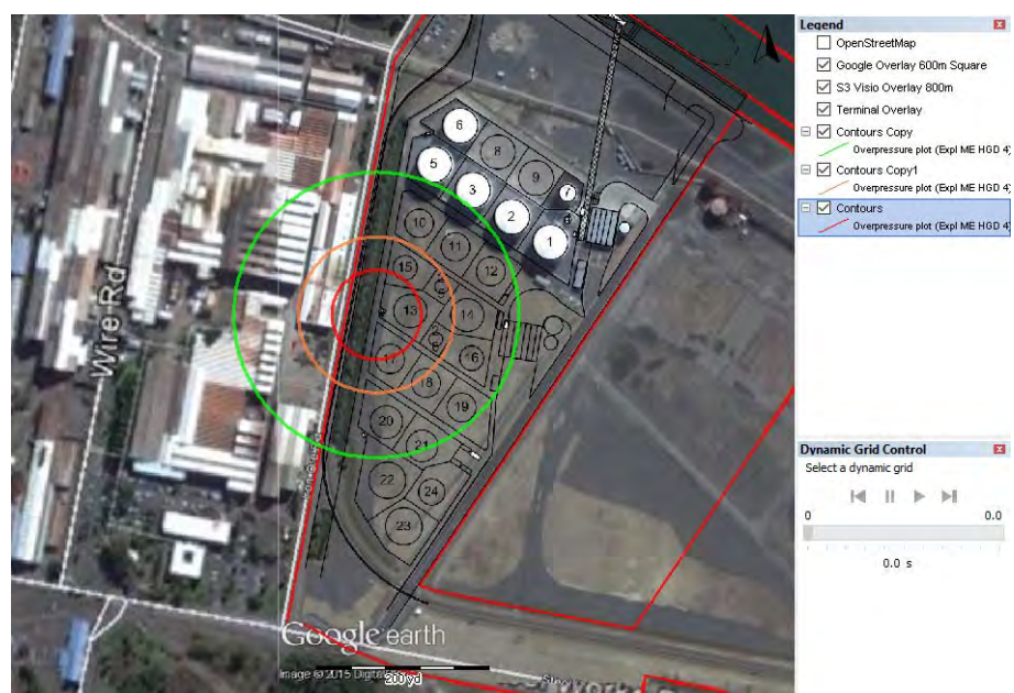
Figure 5 Incident Overpressure Contours – F2.0 Easterly
