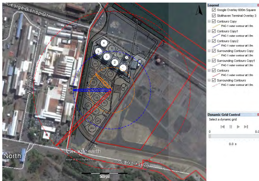
Figure 7 NMA Toxic Dispersion for D5.9, E3.5 and F1.9 atmospheric conditions
