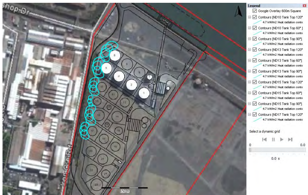
Figure 2 Tank-top fires on western perimeter – heat radiation at 4.7 kW/m 2 at 1.5m height
