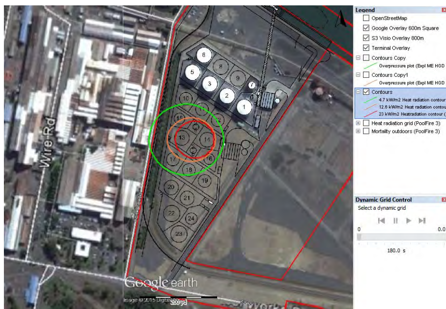
Figure 3 Full Bund Fire - Extent of Heat radiation contours (Easterly wind)
