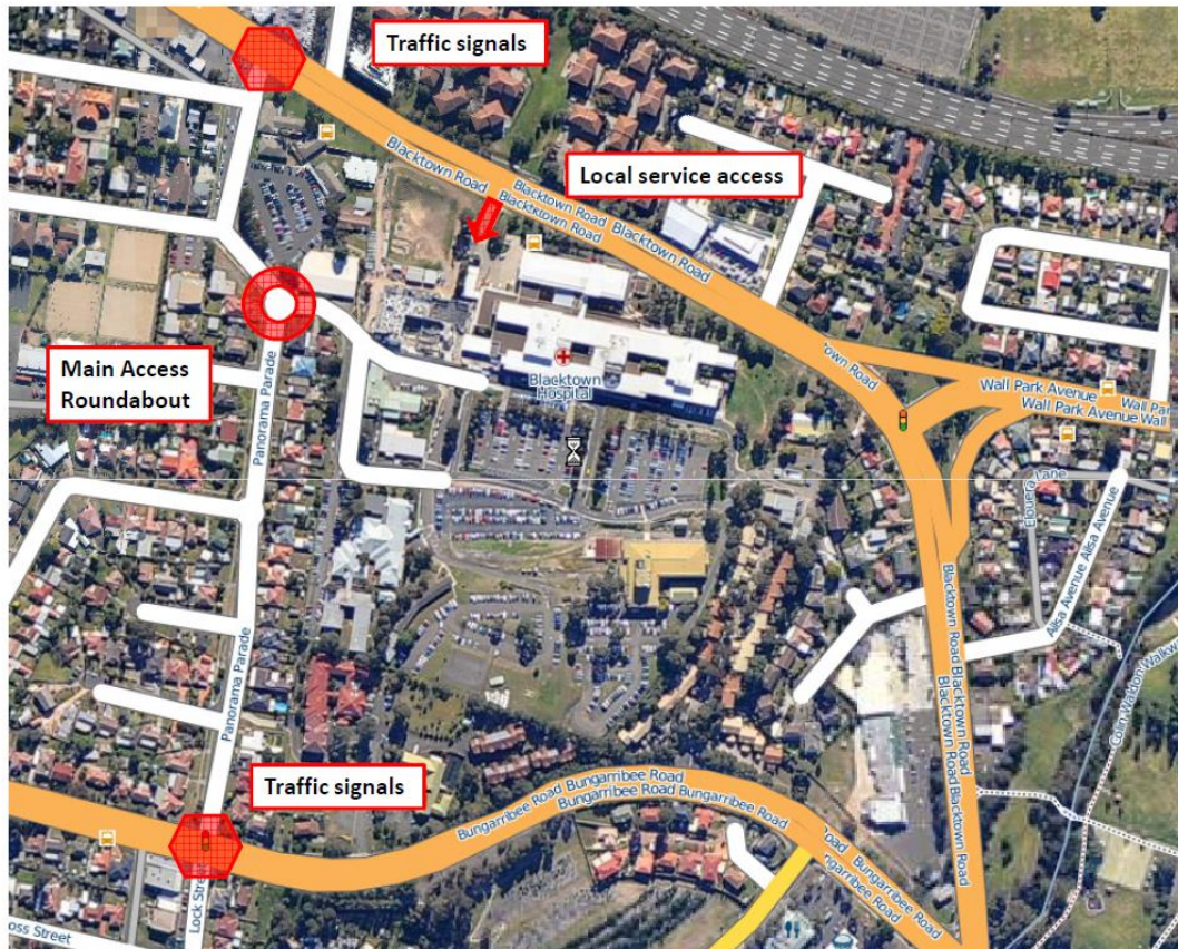
Figure 2 Existing access arrangements and intersection control
