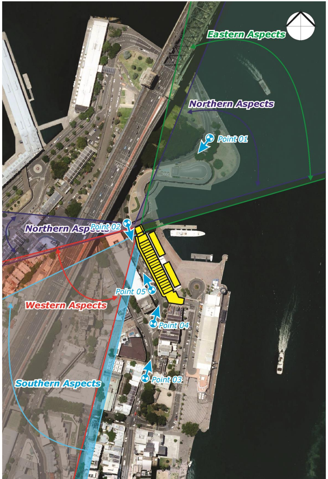
Figure 2a: Check Zones and Study Point Locations for the Main Building Façade of Bay 12 (the check zones are the areas where glare could potentially be observed)
