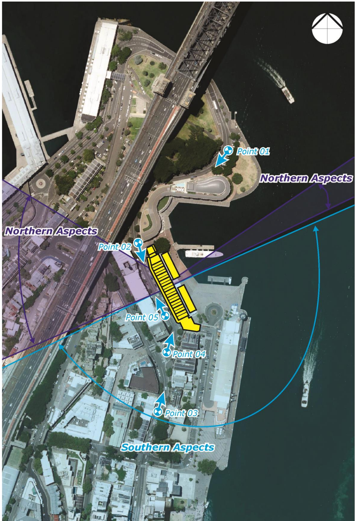
Figure 2b: Check Zones and Study Point Locations for the Skylights on the Bay 6 Roof (the check zones are the areas where glare could potentially be observed)
