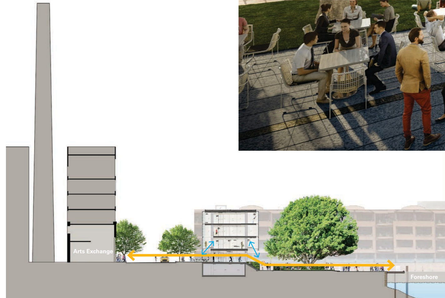
Figure 6.23 Rendered section (NTS) showing the matching height & scale of Bay 12 in relation to the Hyatt, compared to the higher adjacent buildings. Pedestrian connections are enabled under the building (yellow arrow), and visual activation of the undercroft via the obscure glass floor in the undercroft (blue arrows)
