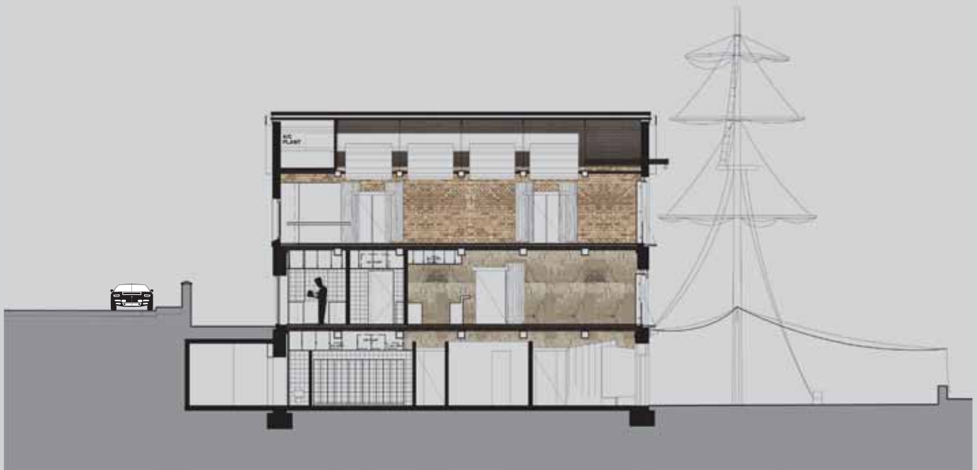
Figure 3.2.1 Existing Cross Section of Typical bay, showing the cluttered service arrangement, finishes, planning and intrusive elements inside and outside the building fabric.
