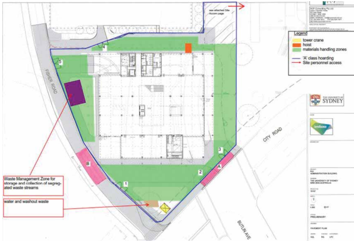
FIGURE 44 – ONSITE WASTE MANAGEMENT/STORAGE LOCATION (SOURCE: LEND LEASE, 2016)
