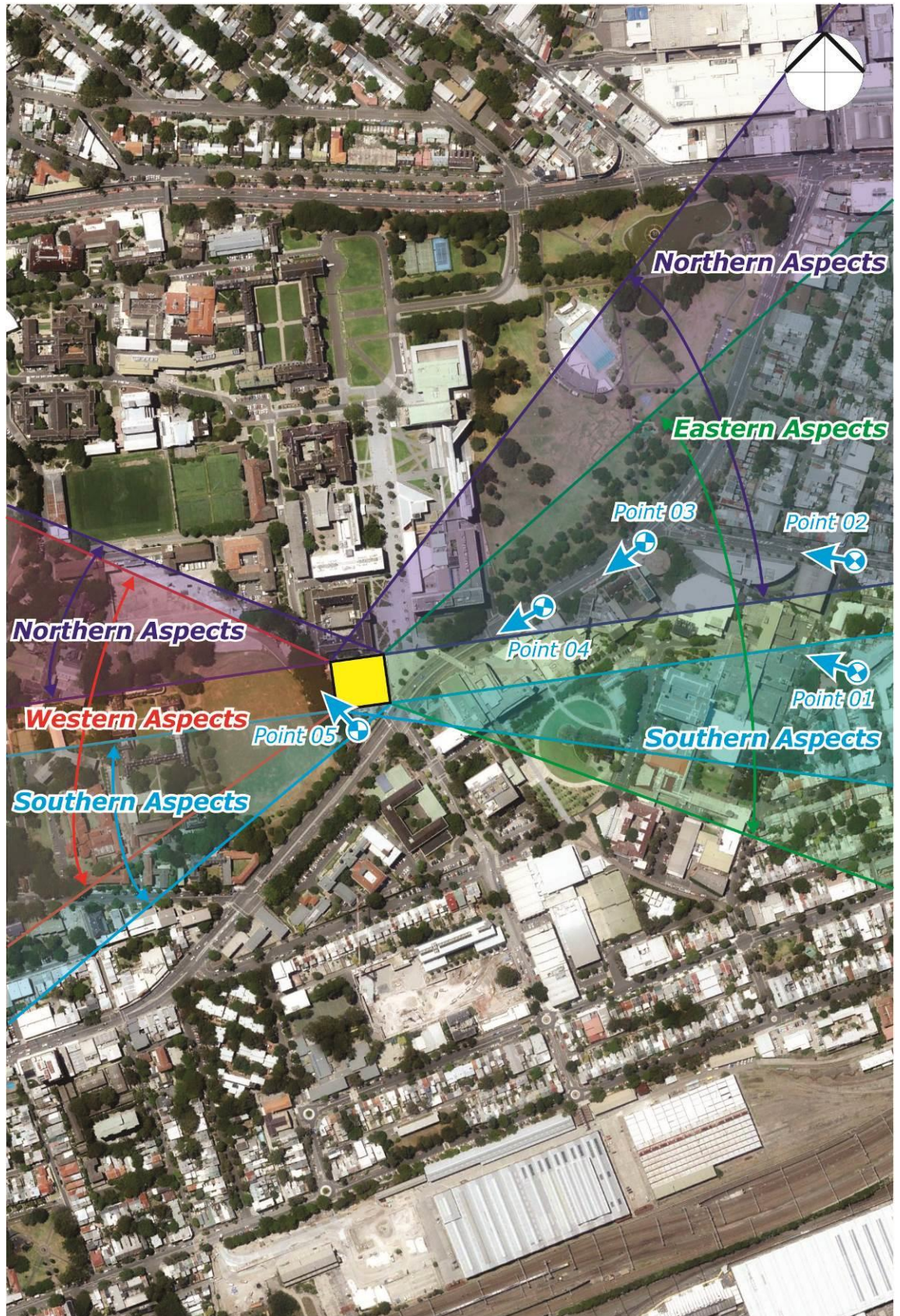
Figure 2: Check Zones and Study Point Locations of the Development (the check zones are the areas where glare could potentially be observed)
