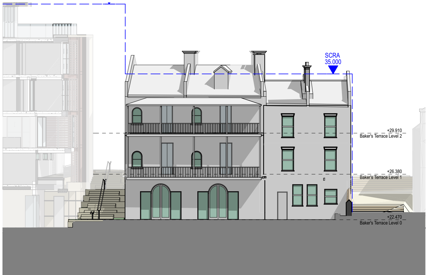
1 ELEVATION East Elevation Outer 1:200 Bakers Terrace
