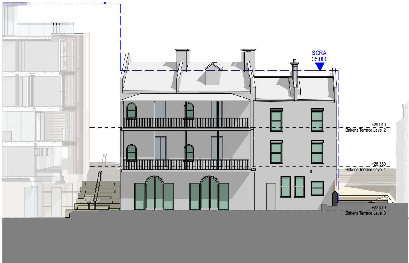
1 ELEVATION East Elevation Outer 1:200 Bakers Terrace
