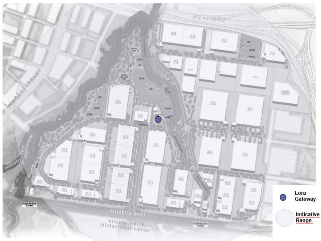
Figure 13: Indicative location for LPWAN antennae and LoRa network coverage
