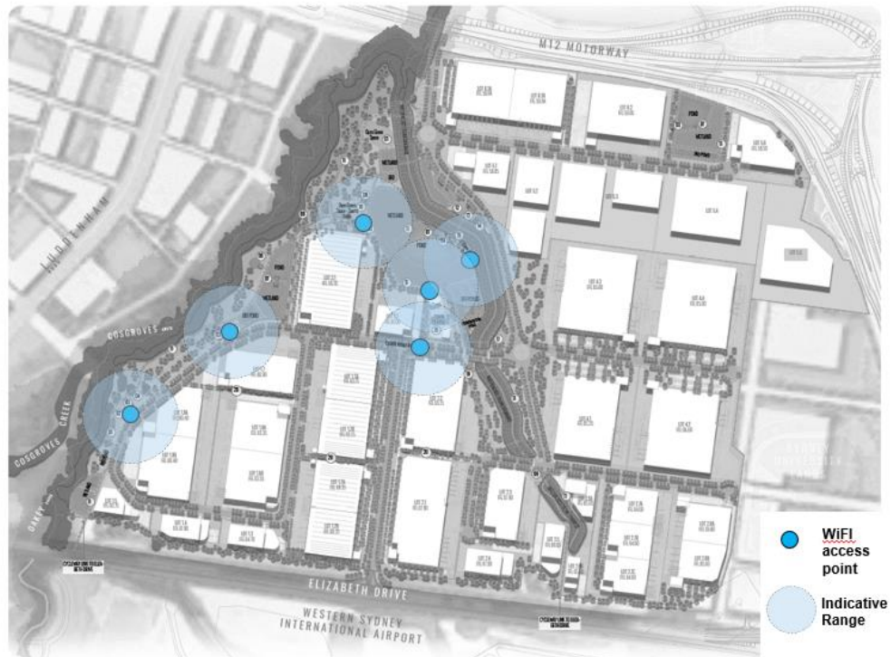
Figure 13: Indicative location for LPWAN antennae and LoRa network coverage
