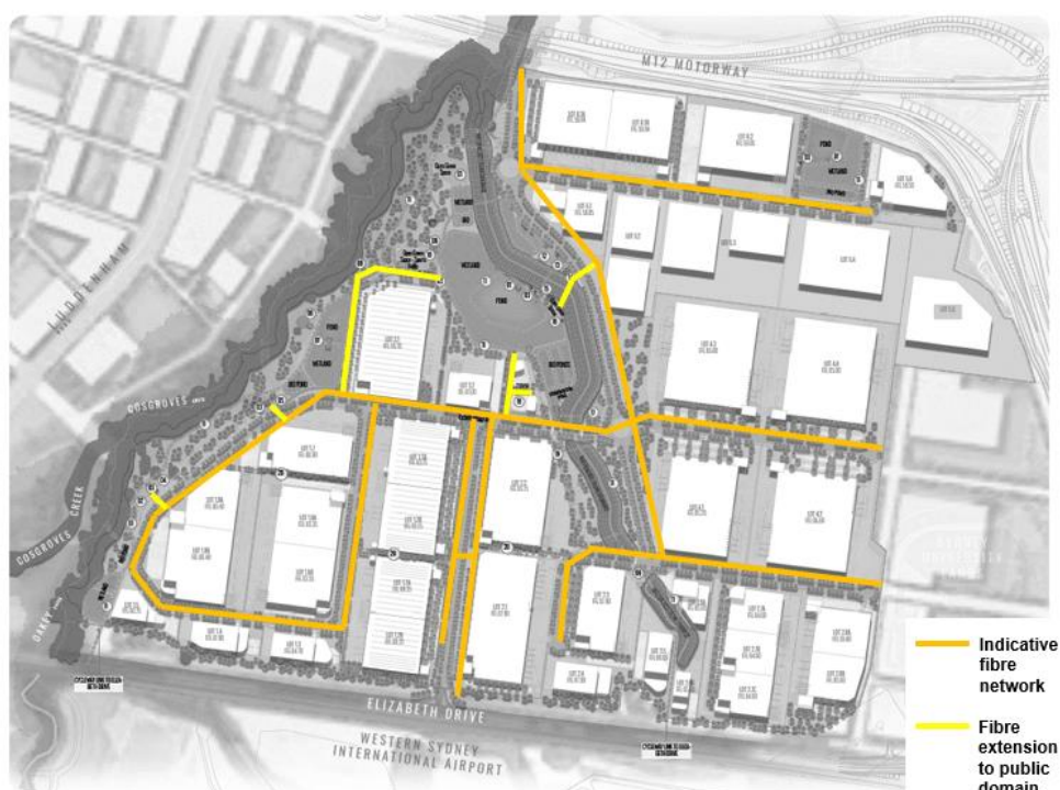
Figure 11: Indicative design for smart city fibre network
