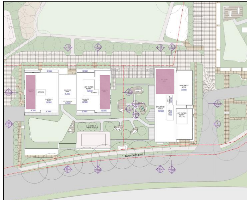
Approximately 140sqm space for PV panels on Building 4 Approximately 196sqm space for PV panels on Building 5
