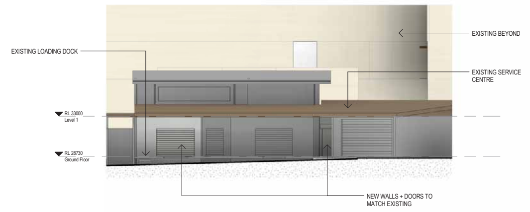
4 Service Centre - East Elevation 1 : 200
