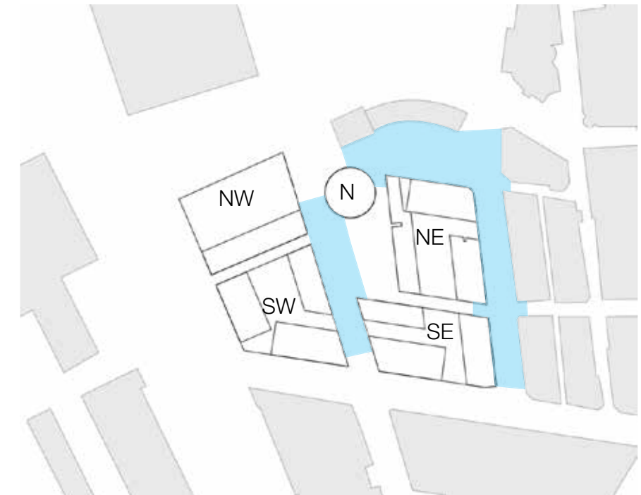
Figure 4.2.3_Overland Flow Diagram Grade separation required to areas shown blue
