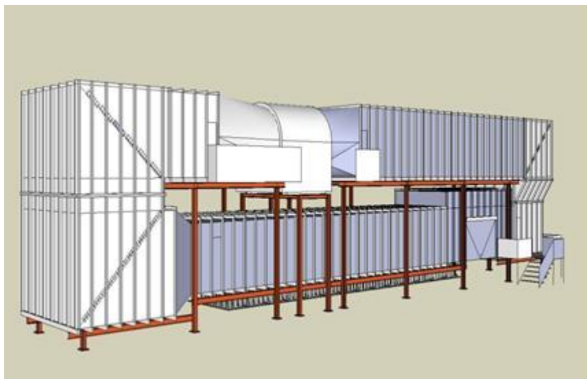
Figure 3: Schematic of the closed circuit wind tunnel
