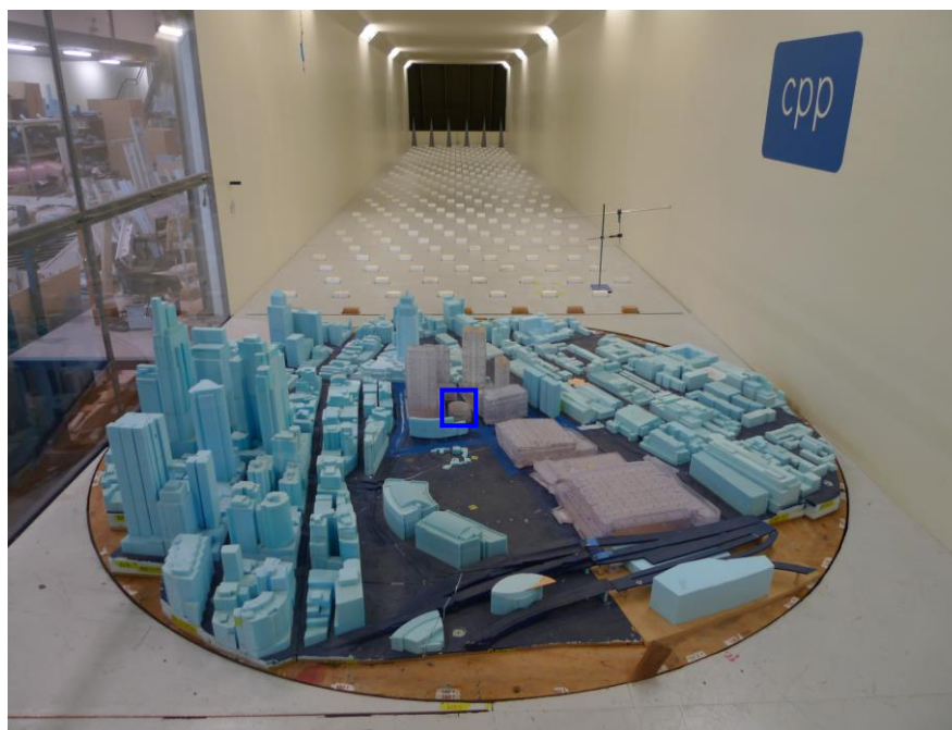
Figure 6: Proposed Darling Square model in the wind tunnel viewed from the north
