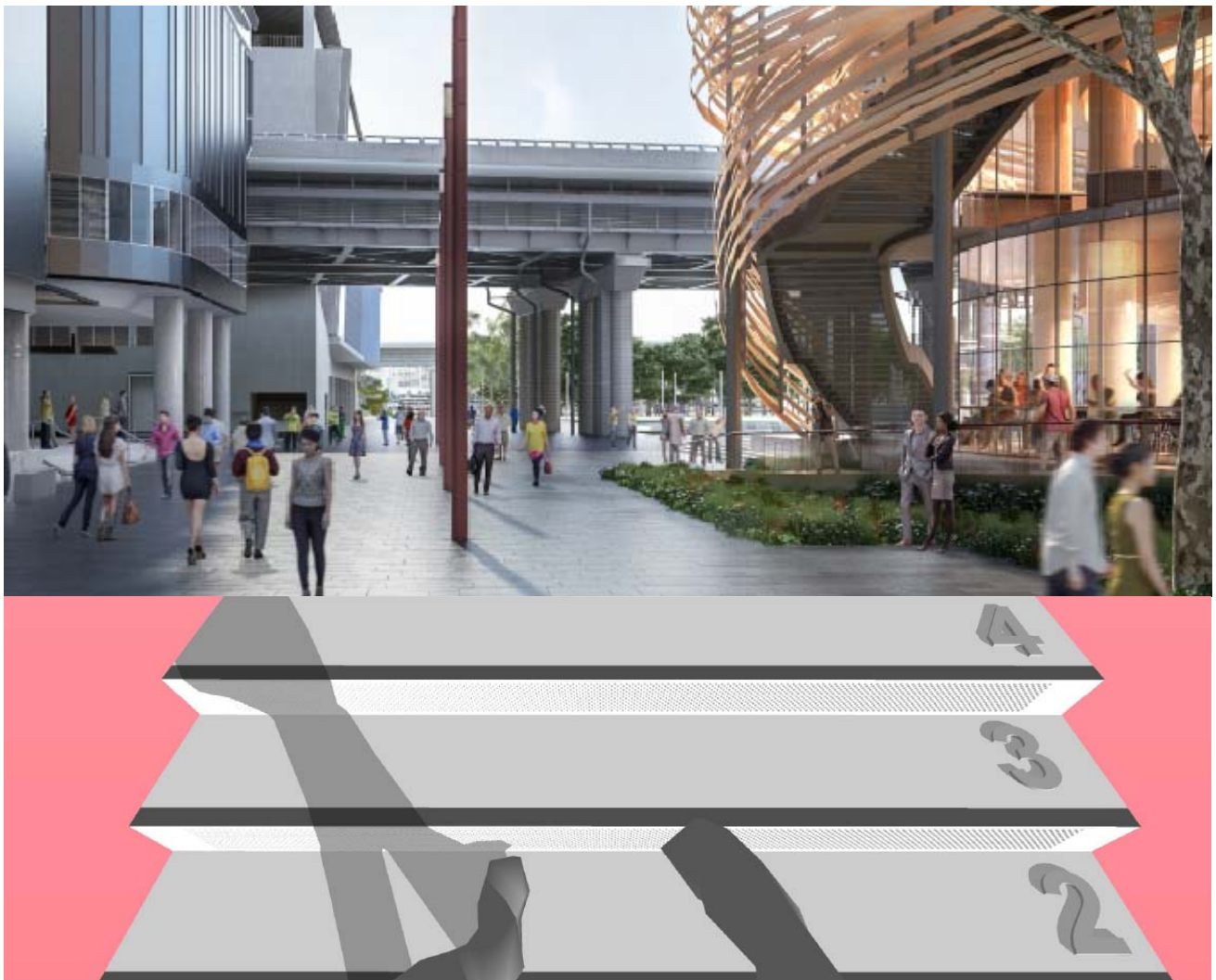
Figure 10: The proposed stair design including 39% stair riser perforation. Computer generated image (top) and image showing level of perforation (bottom) (Source: Applicant's Updated RtS)
