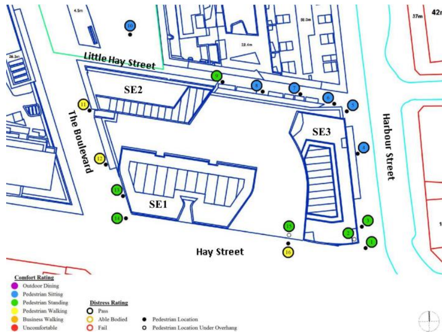
Figure 4: Pedestrian wind speed measurement locations with comfort/distress ratings Little Hay Street
