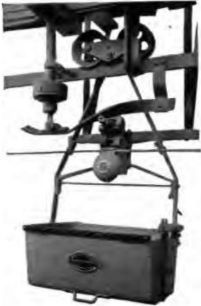
Fig. 9. Carrier, with Webber Patent Compression Grip, showing Patent Automatic Attacher.
