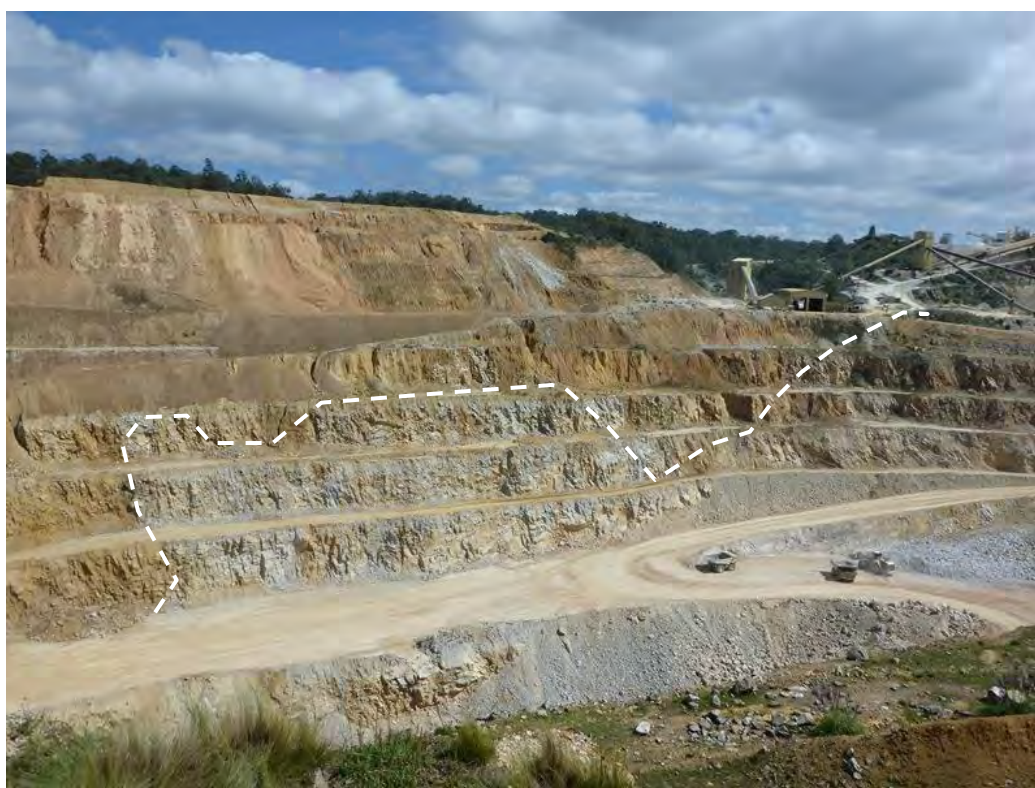
Figure 5-9 Westerly view of hanging wall with weathering profile.
