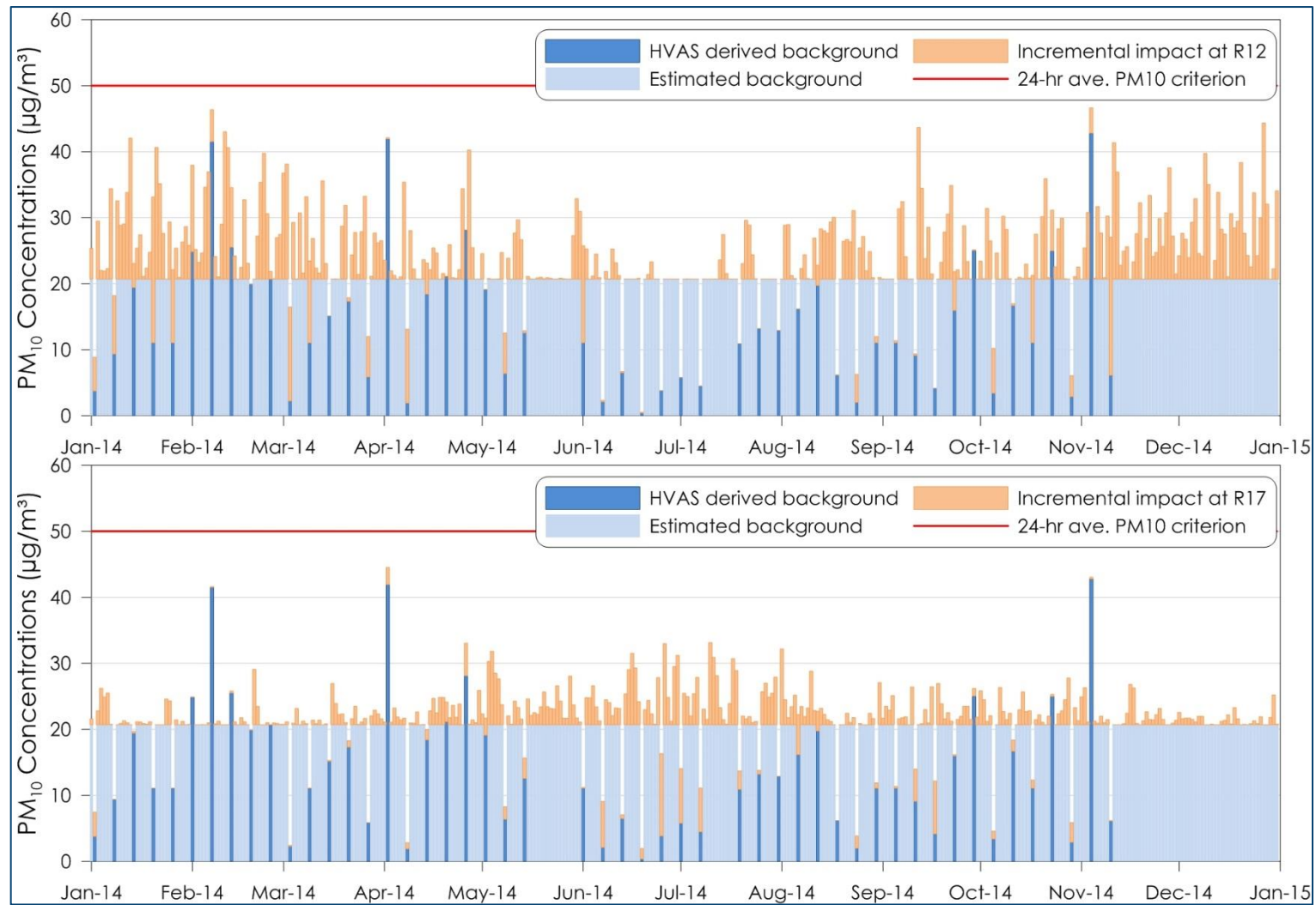
Figure 9-7: Time series plots of predicted cumulative 24-hour average PM 10 concentrations for R12 and R17 – Stage 3
