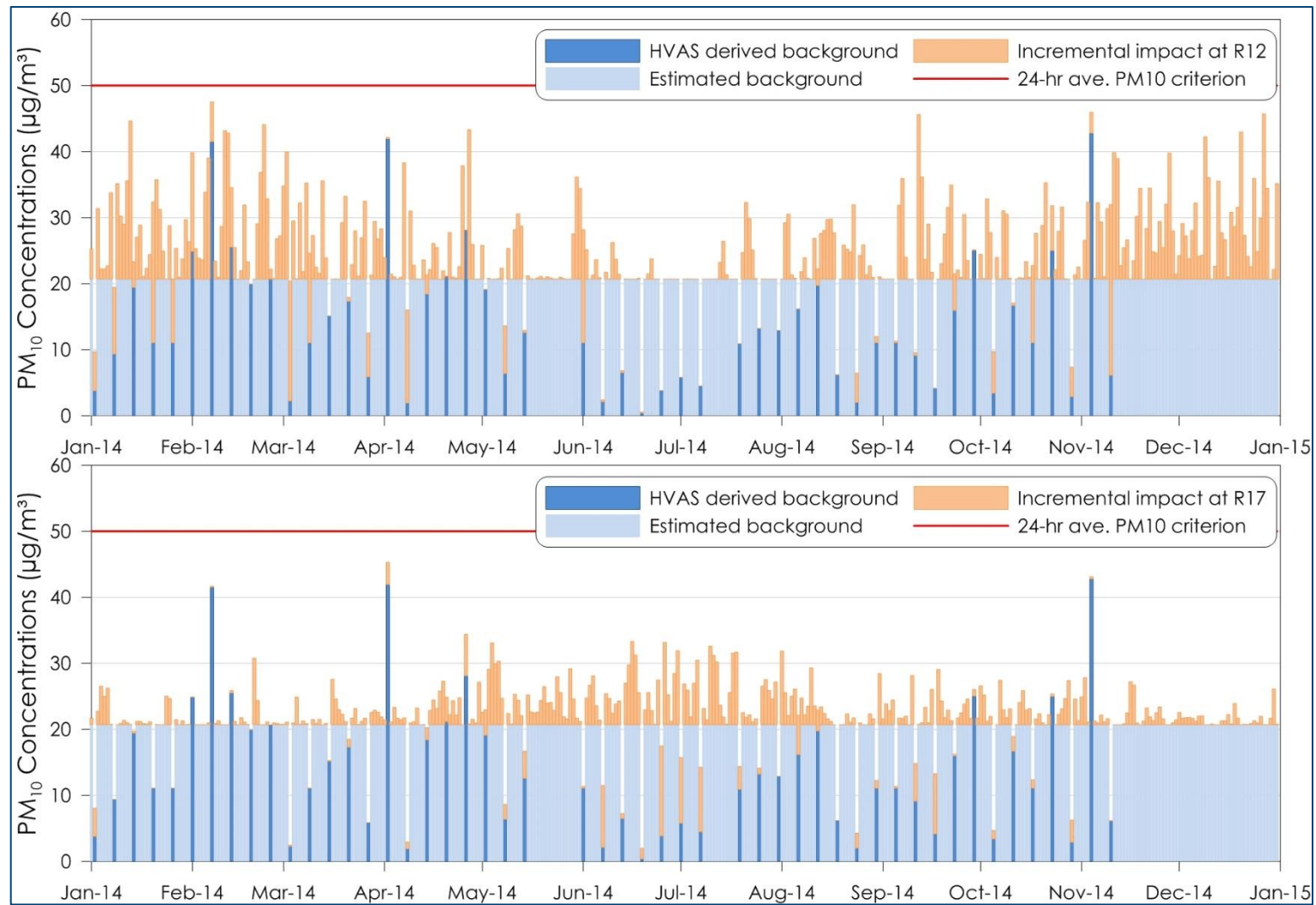
Figure 9-3: Time series plots of predicted cumulative 24-hour average PM 10 concentrations for R12 and R17 – Stage 1
