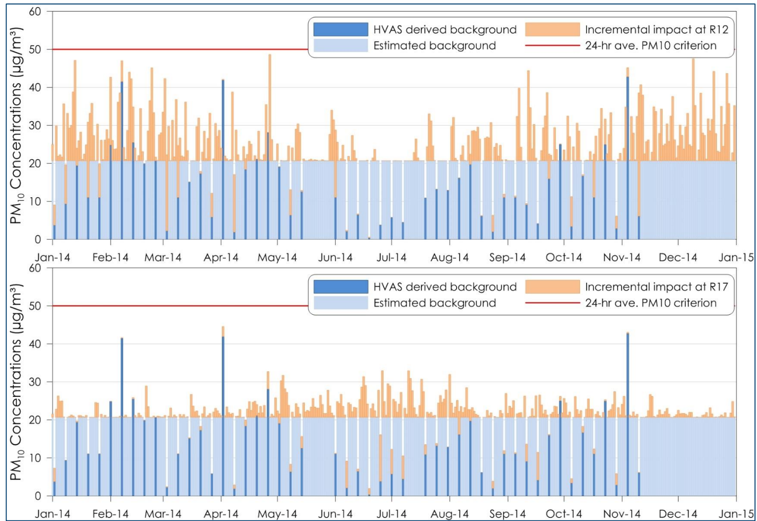
Figure 9-5: Time series plots of predicted cumulative 24-hour average PM 10 concentrations for R12 and R17 – Stage 2
