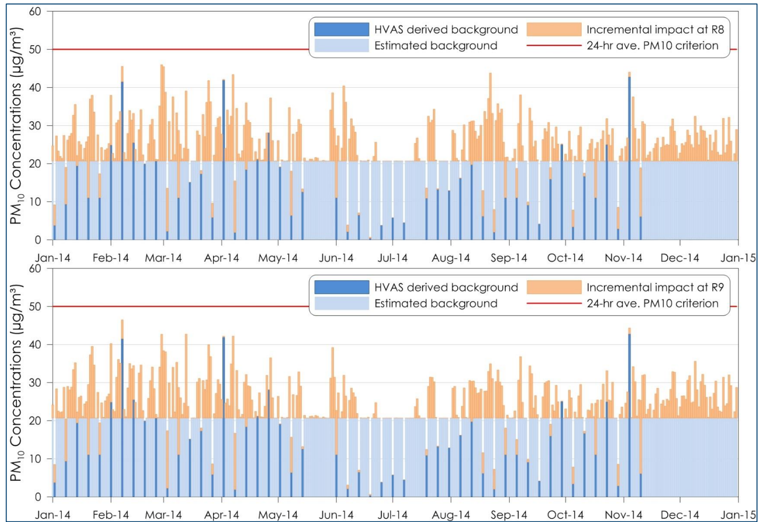
Figure 9-2: Time series plots of predicted cumulative 24-hour average PM 10 concentrations for R8 and R9 – Stage 1
