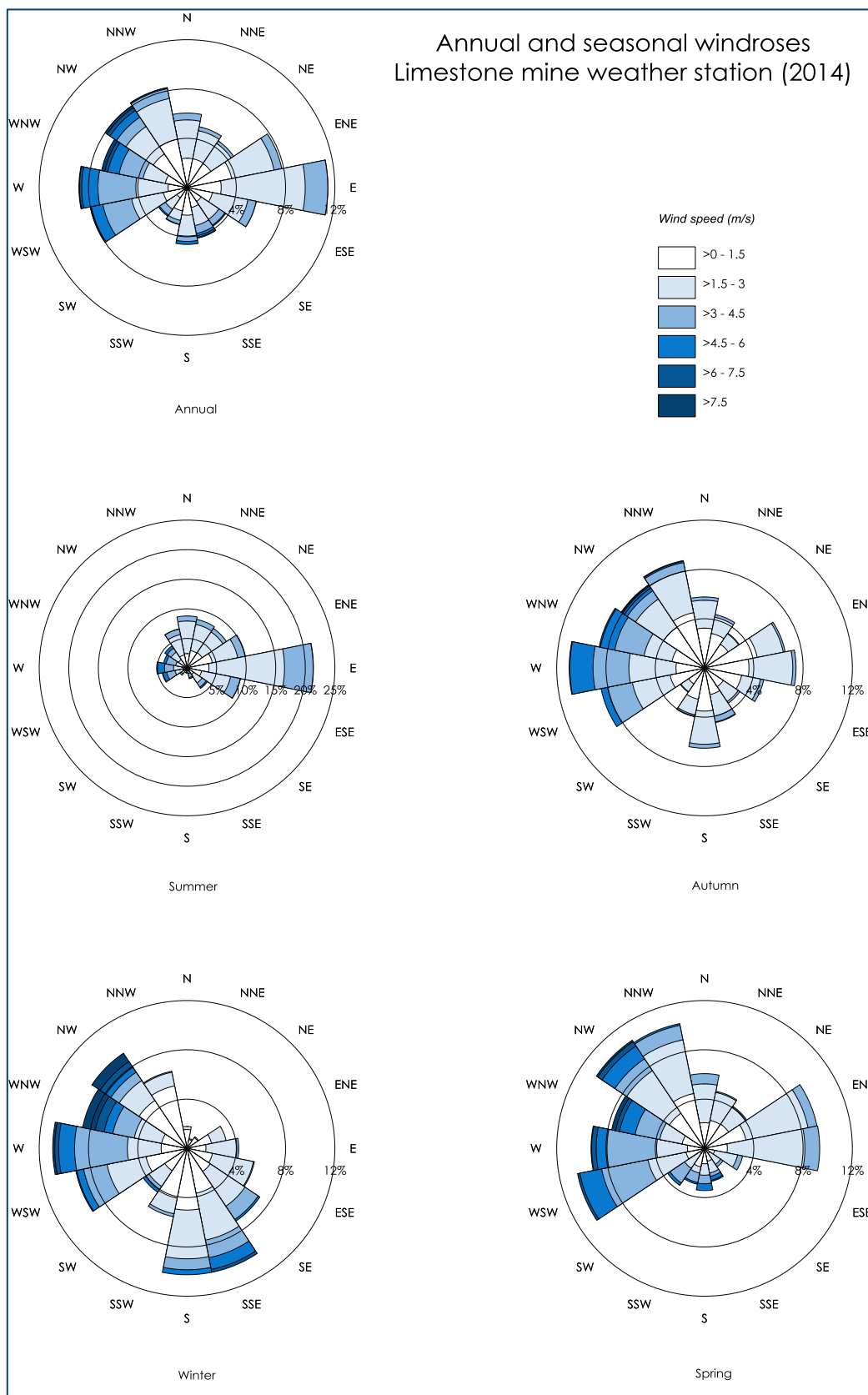
Figure 6-3: Annual and seasonal windroses for the Limestone mine weather station (2014)
