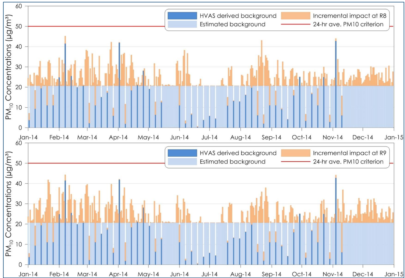
Figure 9-6: Time series plots of predicted cumulative 24-hour average PM 10 concentrations for R8 and R9 – Stage 3
