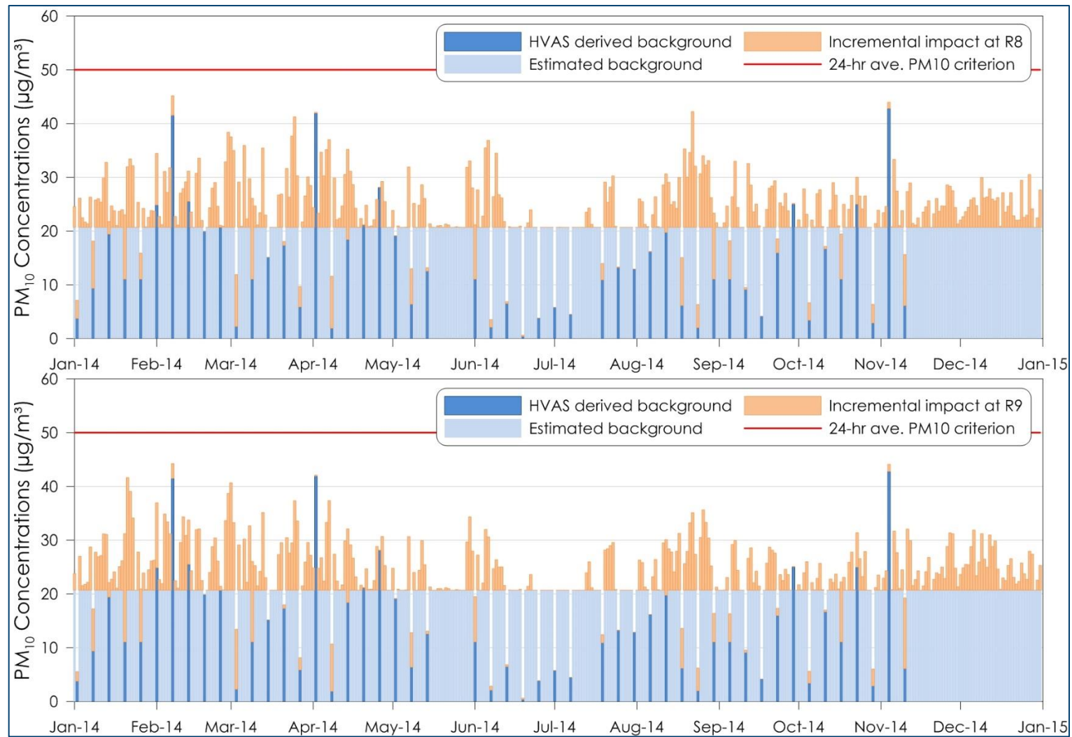
Figure 9-4: Time series plots of predicted cumulative 24-hour average PM 10 concentrations for R8 and R9 – Stage 2
