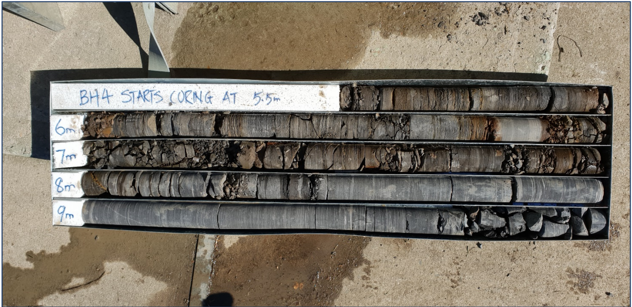
Photograph 1: BH4 upper core showing weathered shale with clay banding.
