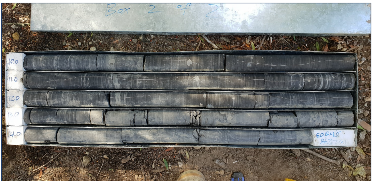
Photograph 4 BH2 lower core showing grey thinly laminated shale.
