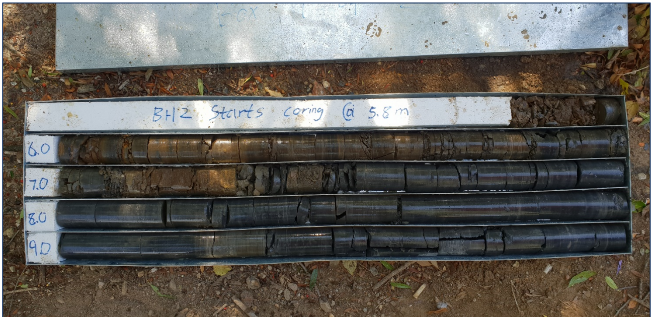
Photograph 3: BH2 upper core showing weathered shale with clay banding.
