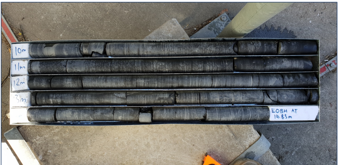
Photograph 2: BH4 lower core showing grey thinly laminated shale.
