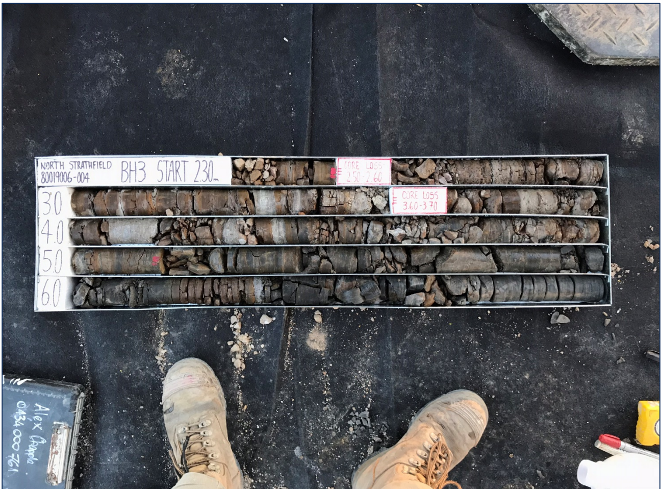
Photograph 6: BH3 core showing orange and brown shale with clay.
