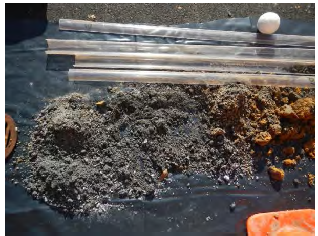
Photo 4 – Ash Fill identified within bore adjacent to potential UST at rear of 624/1 Pittwater Road.
