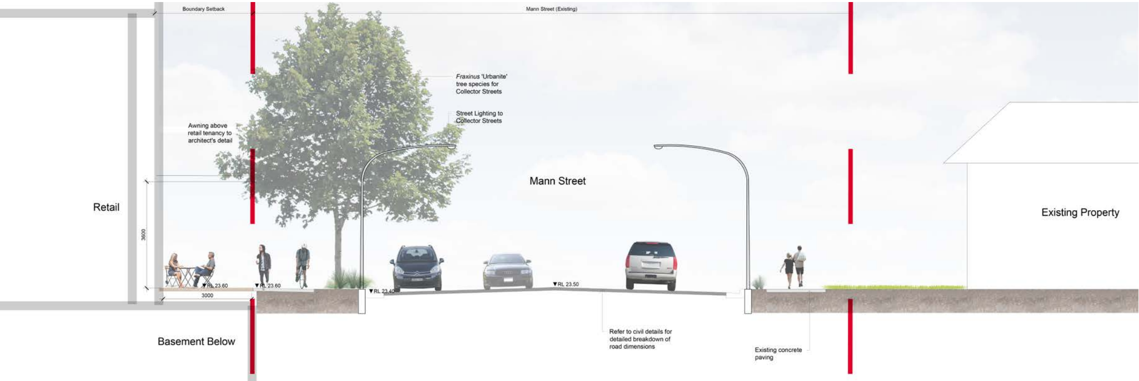
Mann Street - Proposed Site Condition Section A-A
